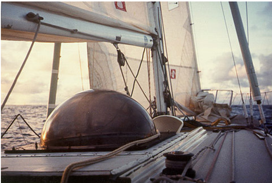
Fig-2 Typical Pacific High weather: Smooth water and a light headwind. Note the dome, the harness tether attached near the mast step, extra ventilator cowls, and anti-chafe gear on the aft lowers.
