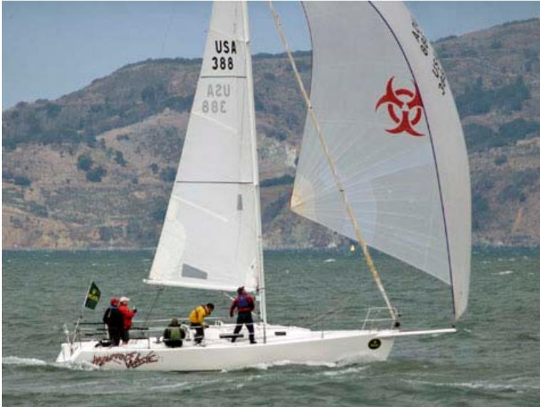
This is a J-105, an example of a sprit boat. The sprit telescopes out from the hull and is limited to pointing straight forward.
